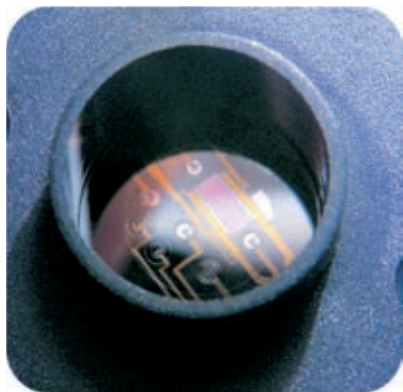
Fig. 2: Silicon sensor chip with sensors for measuring pH and oxygen changes as well as monitoring adhesion.
